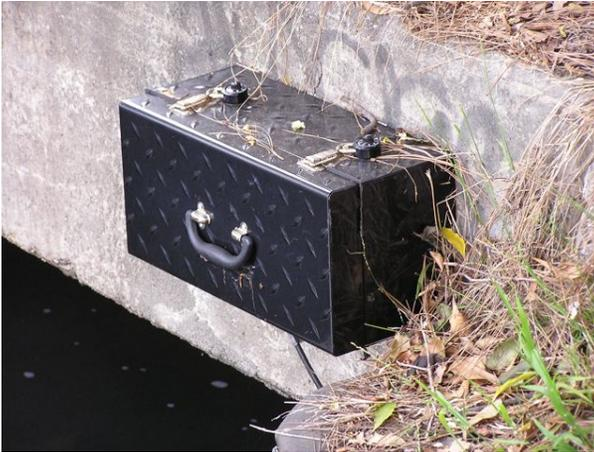
*A new, city stream gage will measure the flow of water in Glen Echo Creek.*
